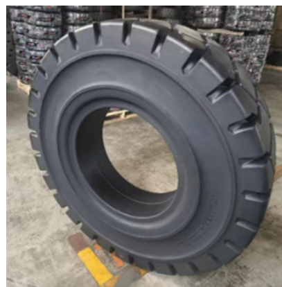
Figure 1 An average resilient solid tyre
