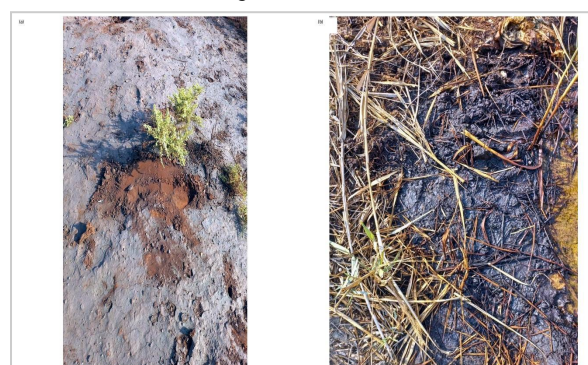
Figure 3. Field evidence of soil and vegetation disturbance: (a) vegetation in an oil-contaminated area; (b) visibly contaminated surface soil.
